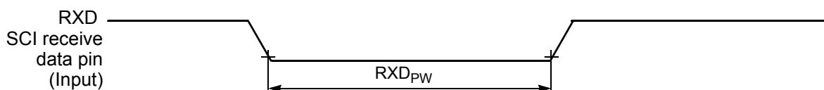
Figure 3-28 RXD Pulse Width
