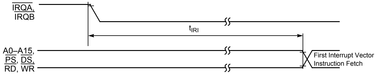
Figure 3-17 Interrupt from Wait State Timing
