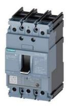
circuit breaker 3VA5 UL frame 125 3-pole, starter protection TM120M, AM, In=100A without overload protection short-circuit protection Ii=5...12 x In cable connection on both sides
