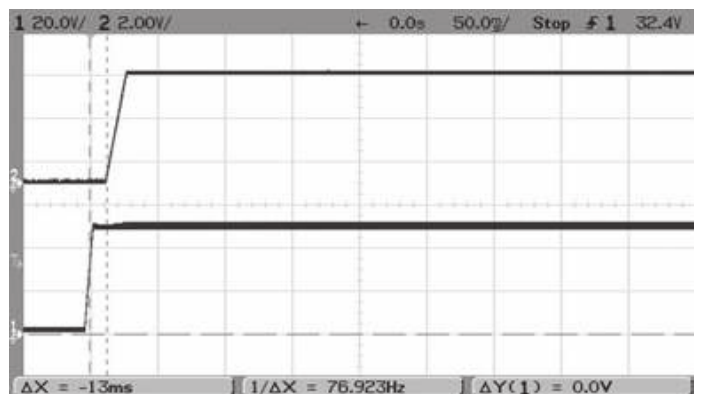
Start-up Delay (Vin = 48V, Vout = nom, Iout = 40A, Cload = 0, Ta = +25°C) ch1 = Vin, ch2 = Vout
