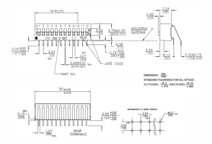
Please find switch body dimensions of 206RA DIP switches with SPDT, DPST, 3PST circuitry on the 206 series data sheet.
