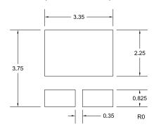
Failure to use this mouning pad layout may result in damage to device.
