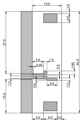
The matching circuit shown has been designed based on the Würth Elektronik evaluation board and cannot be reused. It is recommended to leave a 'Pi' or 'T' type matching circuit space for antenna matching circuit for other boards
