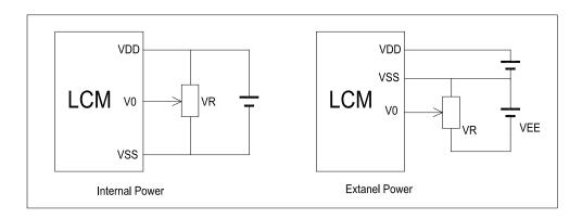
V<sub>DD~</sub>V<sub>0</sub>: LCD Driving voltage
