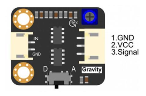
Flexible Piezo Film Vibration Sensor
