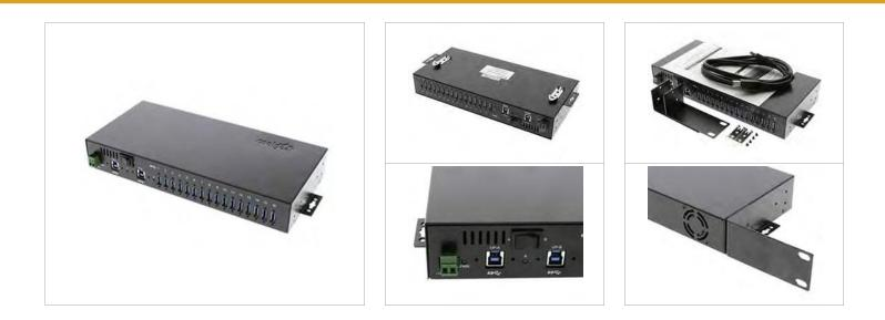
The USB3-16U1 USB 3.0 16 Port USB 3.0 DIN-Rail mounted hub provides an ideal solution for expanding your application by 16 USB 3.0 ports. All ports support Charge and Sync Simultaneously and standard screw lock type USB cables for a secure connection. The 2-Pin self power input connector uses 1 pin for positive voltage and the other pin for a GND connection.
