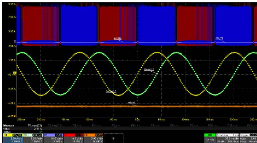
Figure 8-2. 1/16 microstepping at 400 pps with I_{FS} = 3 \text{ A}
