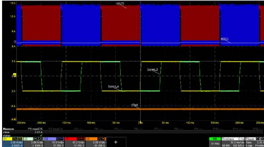
Figure 8-3. Full-step at 25 pps with I_{FS} = 3\text{ A}
