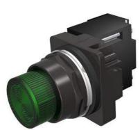
30mm BlackMax, Epoxy Coated Corrosion Resistant Complete Metal Unit Illuminated Indicator Light Full Voltage type, 6V AC/DC Incandescent Lamp, BA9s Plastic Lens, Green UL Listed, CSA Certified NEMA 1,3,3R,4,4X,12,13 & Automotive Standards
