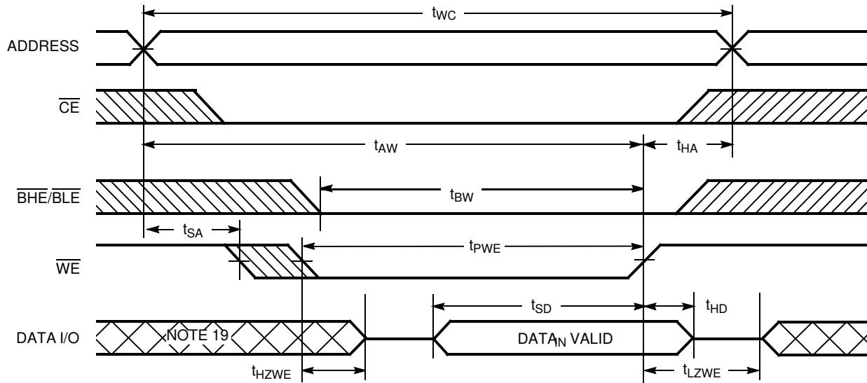
Write Cycle No. 4 ( $\overline{\text{BHE}}/\overline{\text{BLE}}$  Controlled,  $\overline{\text{OE}}$  LOW)<sup>[18]</sup>
