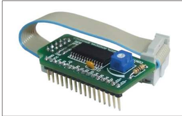
Figure 1: Serial LCD Adapter additional board
