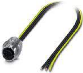
Flush-type connector, Power, 3-position, SocketLink:M12, S power, Front mounting, M16 x 1.5, Individual wires, Cable length: 0.5 m
