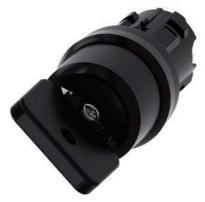
Key-operated switch O.M.R, 22 mm, round, plastic, lock number 73034, black, with 2 keys, 2 switch positions O-I, latching, actuating angle  $90^\circ$ , 10:30h/13:30h, key removal I, with laser labeling, lower case
