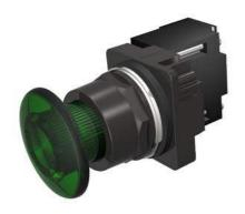
30mm BlackMax, Epoxy Coated Corrosion Resistant Complete Metal Unit Illuminated Push-Pull Operator Transformer type, 120V AC LED Lamp Mushroom Head Cap Small 1 3/4" (44.5 mm) Plastic, Green 2 Position Maintained, Pull-to-Release UL Listed, CSA Certified NEMA 1,3,3R,4,4X,12,13 & Automotive Standards
