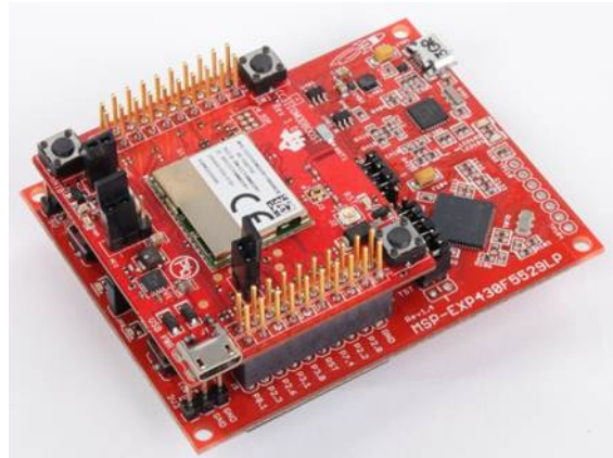
Figure 16. CC3100MODBOOST Connected to MSP430F5529 LaunchPad
