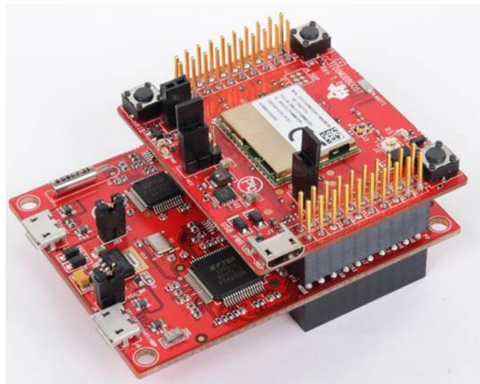
Figure 15. The CC3100BOOST Connected to the EMUBOOST
