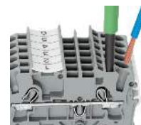
Inserting a conductor via operating tool: Connecting fine-stranded conductors without ferrules, or small cross-sectional conductors that cannot be pushed in, is performed similarly to the original CAGE CLAMP® – just use an operating tool. Advantage: To open the clamp, the operating tool is inserted vertically. The conductor entry is less than 15 degrees for easier wiring.
