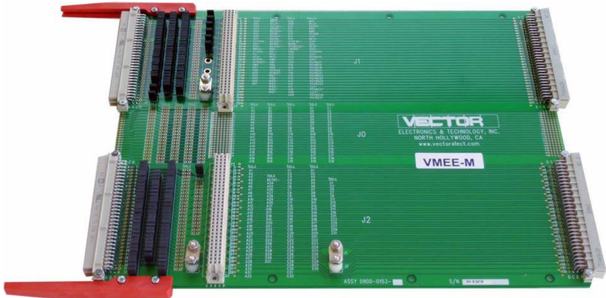
6U VME J1/J2 with 3-row, 96 positions DIN 41612 style connectors ( click on image to enlarge)
