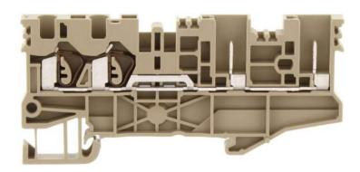
Feed-through terminal, Tension-spring connection, Mounting type: Mounting rail TS 35/7.5, Rated cross-section: 2.5 mm², Width: 5.1 mm, Colour: Beige
