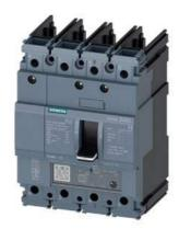
circuit breaker 3VA5 UL frame 125 breaking capacity class M 35kA @ 480V 4-pole, line protection TM230, FTAM, In=100A overload protection Ir=100A fixed short-circuit protection Ii=5...10 x In N conductor unprotected without connection
