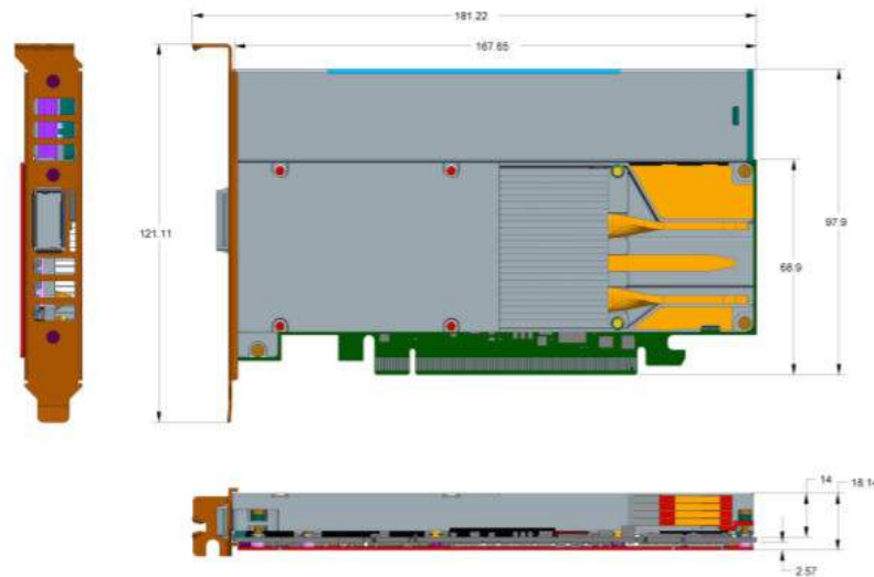
Figure 4. Acceleration Card - Standard Profile Bracket with Airduct
