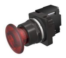
30mm BlackMax, Epoxy Coated Corrosion Resistant Complete Metal Unit Illuminated Push-Pull Operator Transformer type, 120V AC LED Lamp Mushroom Head Cap Small 1 3/4" (44.5 mm) Plastic, Red 3 Position Pull-Momentary/Push-Maintained UL Listed, CSA Certified NEMA 1,3,3R,4,4X,12,13 & Automotive Standards
