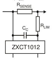
If large reverse currents are expected then the resistor, R<sub>LIM</sub>, will provide protection from exceeding absolute maximum ratings.
