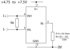
Measuring a current from a circuit which is floating with respect to the DPM's supply, i.e. the current and the meter's power supply are isolated from each other. Ensure solder link LCOM is closed.
