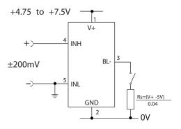
Measuring a single ended input voltage referenced to supply, i.e. the input voltage and the meter's power supply share the same OV rail. Ensure solder link LCOM is open.
