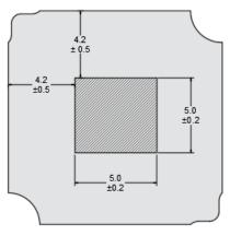
Tc measurement point: either the anode or cathode solder pad
