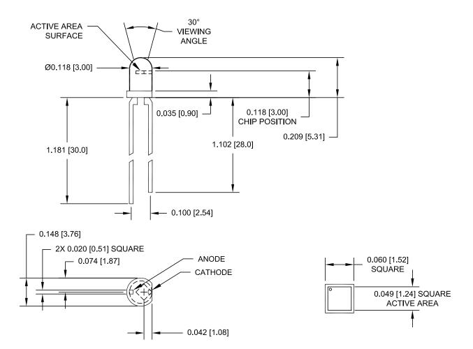
Soldering Conditions:  $260\,^{\circ}\text{C}$  1/16 inch away from case for 3 seconds max.
