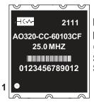
Date Code (YYWW) Model Number Output Frequency Serial # Barcode Serial Number
