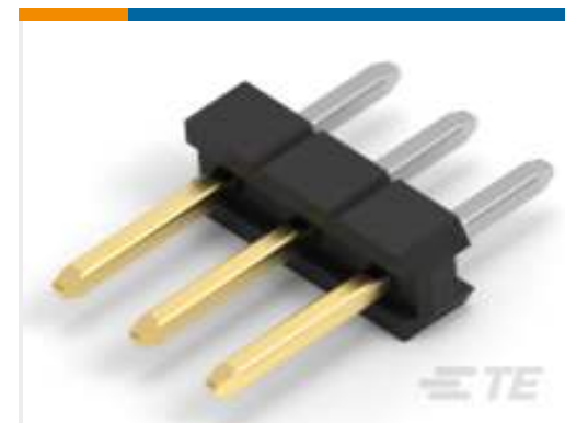
TE Part #2355181-4 4P, 2MM, BRK HDR, SRVT, 2.8, 0.38AU, BOX
