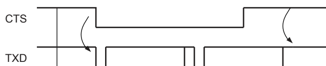
Figure 36-28: Transmitter Behavior when Operating with Hardware Handshaking
