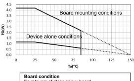
Four layers of glass epoxy board Cu thickness: 1-layer/4-layer=55mm, 2-layer and
