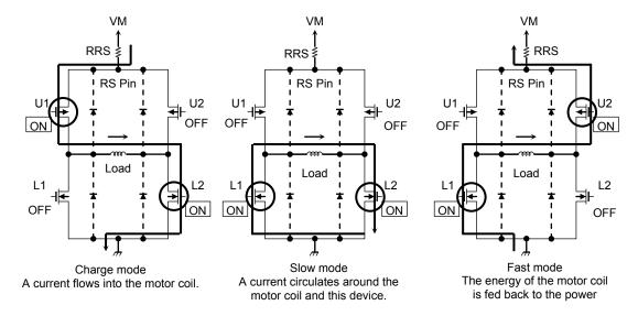
**Output transistor operational function**
