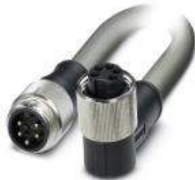
Bus system cable, DeviceNet, 5-position, PVC, Gray RAL 7001, Plug straight 7/8"-16UNF, on Socket angled 7/8"-16UNF, Cable length: 2 m
