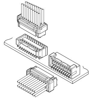
In order to correspond to the high-density PC board designing, this ZPD connector is designed as 1.5mm pitch double row type connector with secure locking device. Low insertion force is realized and good mating feeling is also prepared, and these provide the certain mating operation.
