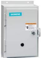
Reversing NEMA contactor Size 1 Three phase full voltage Contactor amp rating 27Amp 3 w 110-120/220-240VAC 60HZ coil Non-combination type Enclosure NEMA type 12 Dust/drip proof for indoors Standard width enclosure
