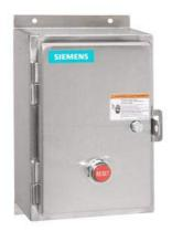
Non-reversing motor starter, Size 3, Three phase full voltage, Solid-state overload relay, OLR amp range 25-100A, 208VAC 60Hz coil, Non-combination type, Encl. type 4X 304 S. Steel, Water/dust tight noncorrosive, Standard width enclosure
