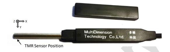
The USB magnetometer hardware is compatible with the popular open source Arduino UNO board, and thus with the Arduino programming environment or Atmel microcontroller development tools. The user may develop custom firmware at his/her own risk. The hardware includes a boot loader for uploading Arduino code. The USB magnetometer hardware model is defined as follows:
