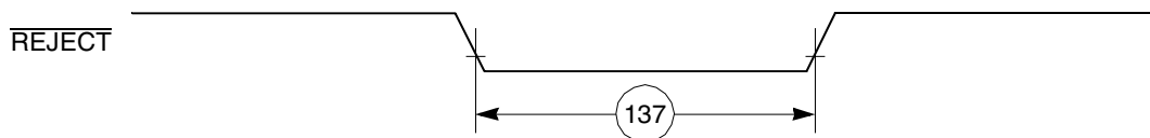
Figure 58. CAM Interface \overline{\text{REJECT}} Timing Diagram
