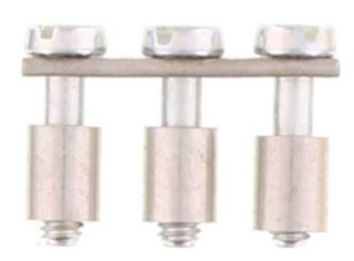
Cross-connector, No. of poles: 3, Mounting type: Can be screwed on, Width: 16.6 mm, Rated cross-section: 2.5 mm², Colour: natural
