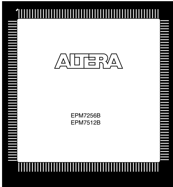
Figure 27. 208-Pin PQFP Package Pin-Out Diagram
