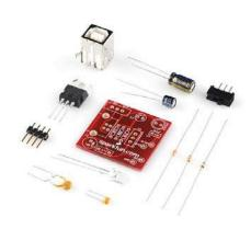
**Description:** A very simple breadboard power supply kit that takes power from any USB port and outputs a fuse protected and regulated 3.3V. The .1" headers are mounted on the bottom of the PCB for simple insertion into a breadboard. Pins labeled 5V/GND 3.3V/GND plug directly into the power lines.
