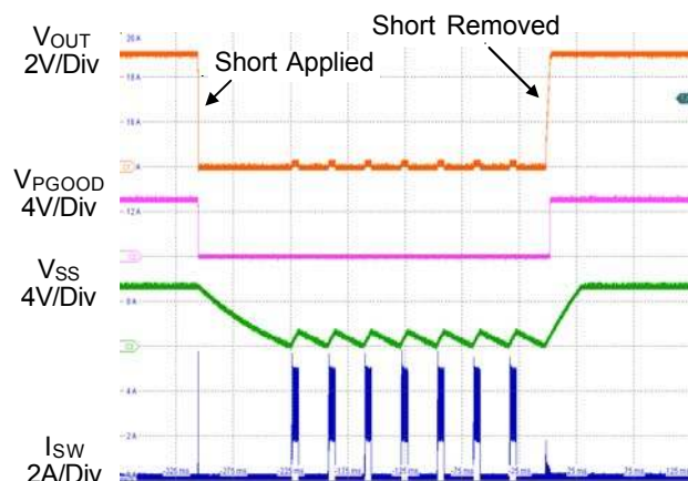
Figure 3. Short Circuit Protection and Recovery
