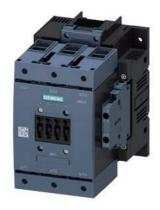
power contactor, AC-3e/AC-3 115 A, 55 kW / 400 V, AC (50-60 Hz) / DC Uc: 240-277 V 3-pole, auxiliary contacts 2 NO + 2 NC drive: conventional main circuit: box terminal control and auxiliary circuit: screw terminal
