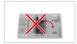
②Insert the FFC correctly into the opening, failing to do so can lead to disconnection or conduction failure.
