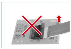
Be careful not to scrape the FFC on the housing of the connector during insertion, this action can lead to damaged contacts, terminal deformation, FFC conductor defects and other failures.
