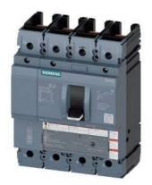
circuit breaker 3VA5 UL frame 250 breaking capacity class H 65kA @ 480V 4-pole, line protection TM230, FTAM, In=70A overload protection Ir=70A fixed short-circuit protection li=5...10 x In N conductor without connection
