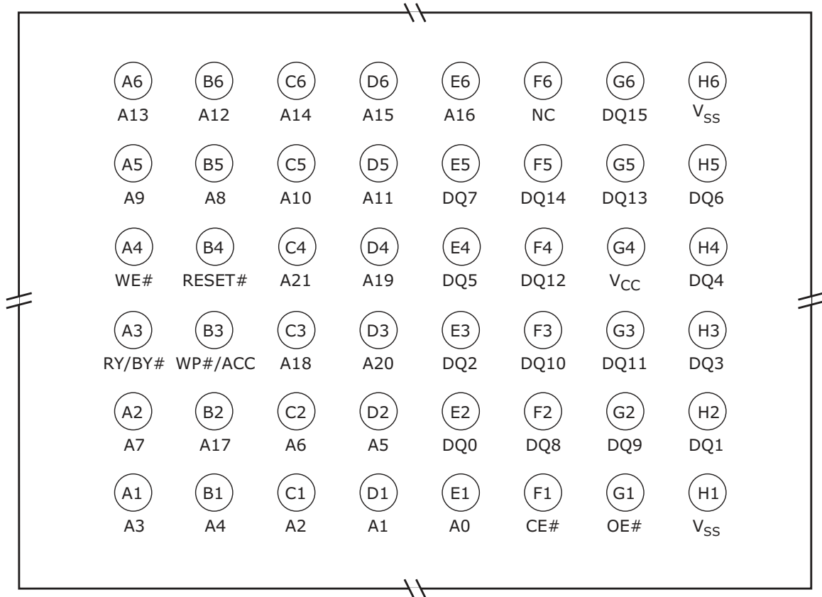
Figure 3. 48-Ball Fine-Pitch BGA, Top View, Balls Facing Down—PL064J—PL032J: C4(A21)=NC
