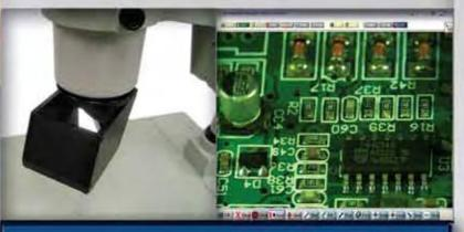
3-D capability: Viewer that attaches easily to the iScope uses a mirror angled at 45 degrees to deliver images with three-dimensional effect.
