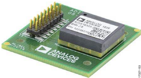
Figure 56. ADIS16500 Breakout Board (ADIS16505-2 Shown)
