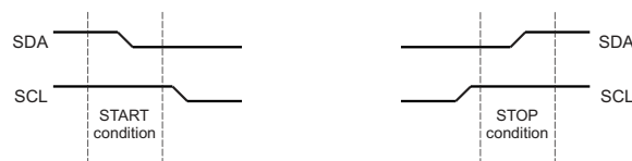
Figure 22-3. START and STOP Conditions
