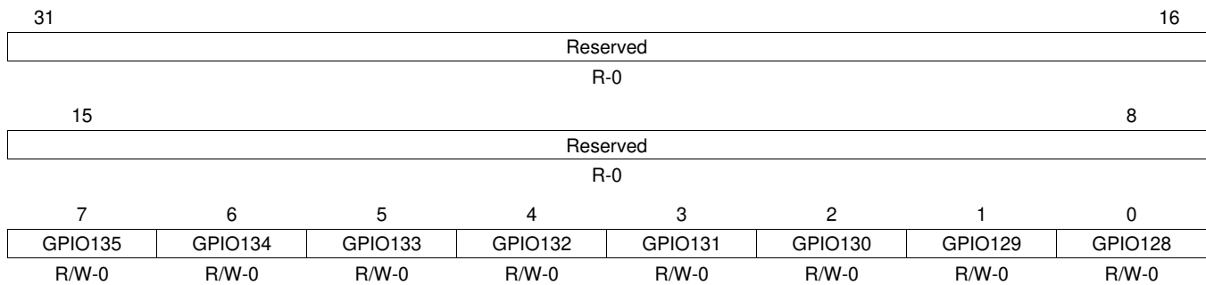
Figure 4-63. GPIO Port E Direction (GPEDIR) Register
