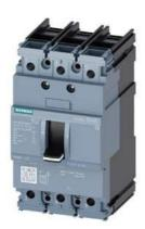
circuit breaker 3VA5 UL frame 125 breaking capacity class H 65kA @ 480 V 3-pole, line protection TM210, FTFM, In=125A overload protection Ir=125A fixed short-circuit protection li=10 x In UL489 SB (naval), 50 deg. cel. cable connection on both sides
