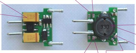
Footprint option allows to test alternative coils, e.g. unshielded option to compare EMI properties (ref. BOM).
