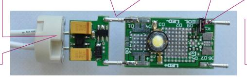
The driver circuit is intrinsically safe against open LED circuit.
