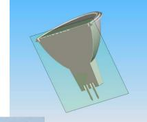
Section of OSRAM Decostar 51 www.osram.com
